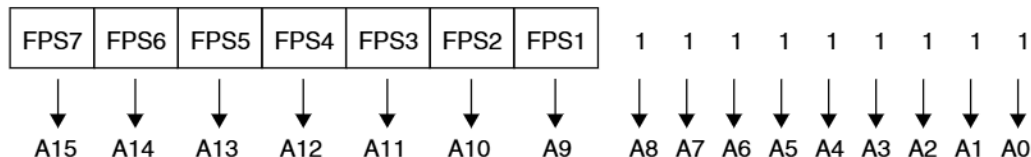
Figure 4-5. Block Protection Mechanism
