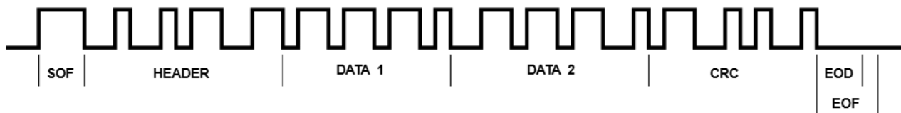
FIGURE 3. TYPICAL J1850 VPW MESSAGE FRAME
